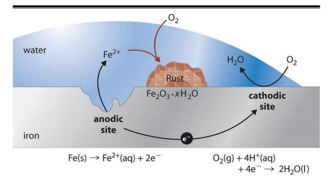
Rusting "applies to the corrosion of iron or iron - base alloys with formation of corrosion products consisting largely of hydrous ferric oxides. Nonferrous metals, therefore, corrode, but do not rust.
