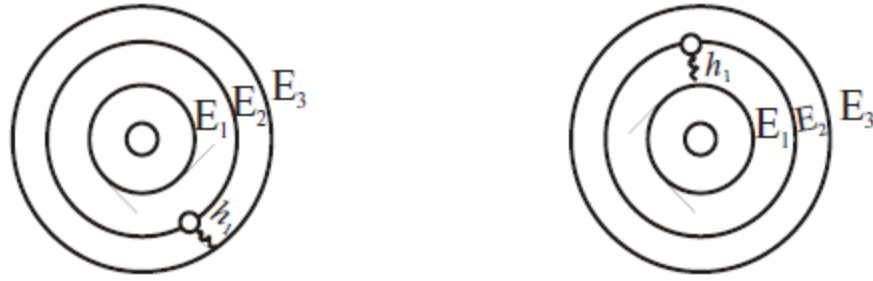
Fig. 7 : Absorption and emission of photon causes the electron to change its energy level.
