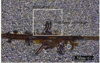
The line in the center represents the knife-score. The filiform corrosion grew in both directions from the line and is composed of a head and the tail. The head and the tail are filled with a  $FeCl_2$  solution and corrosion products, respectivel.
