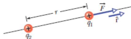
Figure 3: The electrostatic force on particle 1 can be described in terms of a unit vector along an axis through the two particles, radially away from particle 2.
