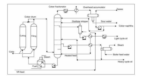
Steam is injected in the furnace to prevent premature coking. The feed to the coker drums is heated to just above 482 °C (900 F). The liquid–vapour mixture leaving the furnace passes to one of the coking drum. Coke is deposited in this drum for 24 h period while the other drum is being decoked and cleaned. Hot vapors from the coke drum are quenched by the liquid feed. Vapors from the top of the coke drum are returned to the bottom of the fractionator.
