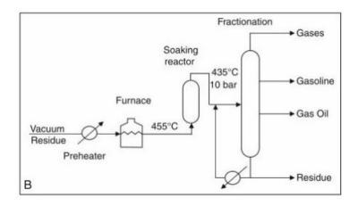
Both process configurations have their advantages and applications. Coil cracking yields a slightly more stable visbreaker product, which are important for some feedstocks and applications. It is generally more flexible and allows the production of heavy cuts, boiling in the vacuum gas oil range. Soaker cracking usually requires less capital investment, consumes less fuel and has longer on-stream times.
