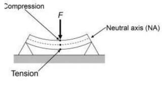
Simple supported beam bending
