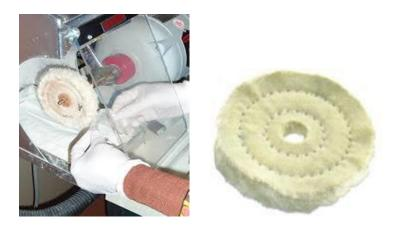
2. Polish acrylic around the teeth with wet pumice and a brush wheel attached to dental lathe moving at slow speed. Be careful not remove previously developed contours.
