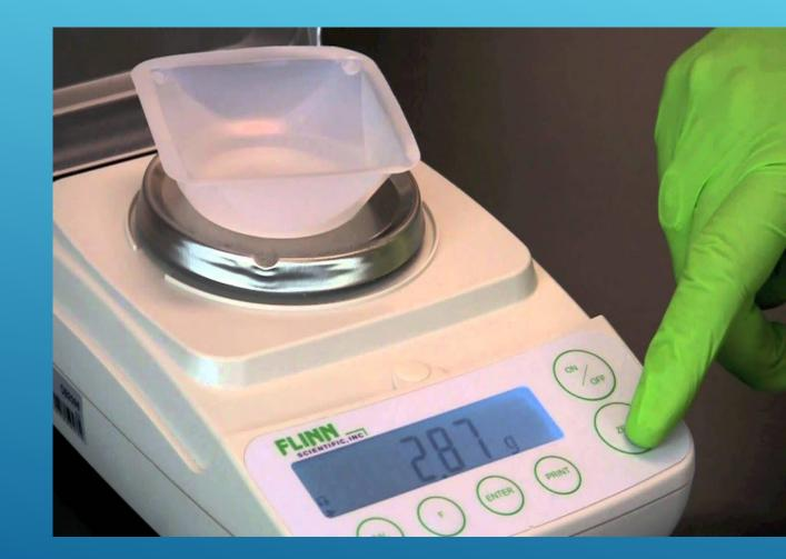
4- Press the "Tare" or "Zero" button to automatically deduct the weight of the container from future calculations. The digital display will show zero again, indicating that the container's mass is stored in the balance's memory.
