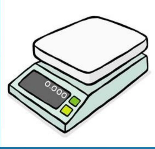
2- clean the surface of the balance before using because Fingerprints and other greases from your hands add mass and must be avoided for accurate measurements. , then Press the "ON" button and wait for the balance to show zeroes on the digital screen.
