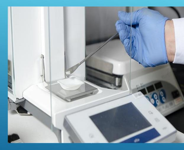
5- Place the container with the substance back on the balance platform if necessary and record the mass as indicated by the digital display. Then you must press ( OFF) button to shut down the device .
