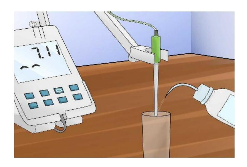
Once you've placed the electrode in the buffer, press the "measure" or " calibrate" It should take 1 to 2 minutes for the pH to stabilize. button to begin reading the pH.At this time, set the pH meter to the value of the buffer's pH by pressing the . "measure" button again
