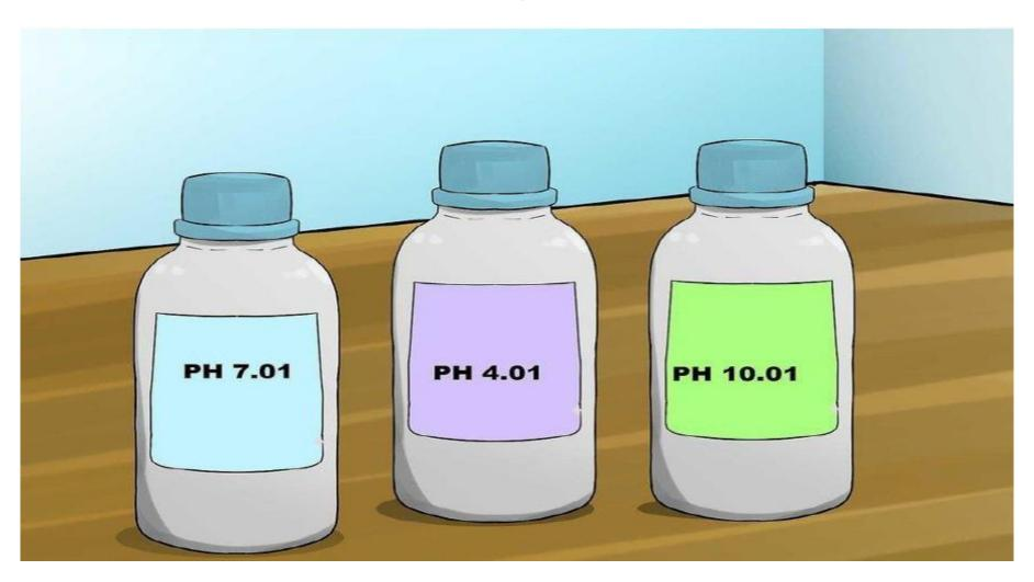
Your first buffer should be neutral, meaning it has a pH of 7. Your second buffer will either have a pH of 4 (for an acidic sample) or 9.21 (for a basic sample).
