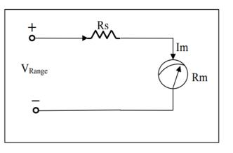
So the internal resistance of voltmeter or the input resistance of voltmeter is
