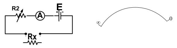
c) Shunt Ohmmeter:
