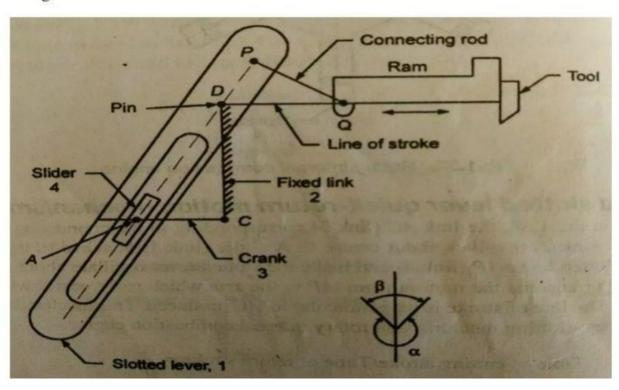
When one of the links of a kinematic chain is fixed, the chain is known as mechanisms. It may be used for transmitting or transforming motion, There are two types of it:a) Simple Mechanism: A mechanism with four links is known as simple mechanism.
