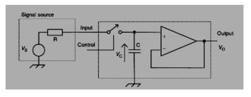
The switch closes only when that particular channel is to be sampled. If the source impedance  $\mathbf{r}$  is small, the capacitor voltage changes to the input voltage within the time  $\tau$  that switch is closed.
