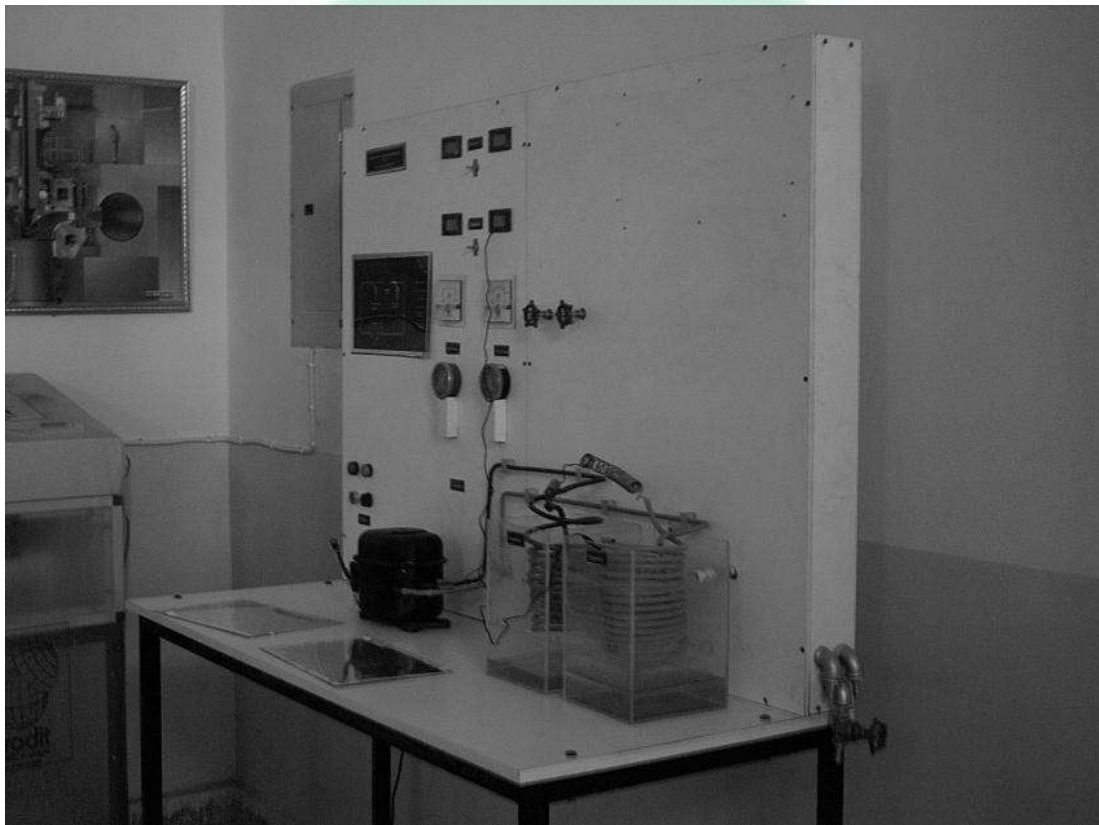
photograph A simple heat pump unit
