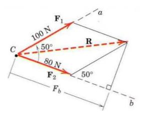
Solution. The parallelogram addition of  $F_1$  and  $F_2$  is shown in the figure. Using the law of cosines gives us
