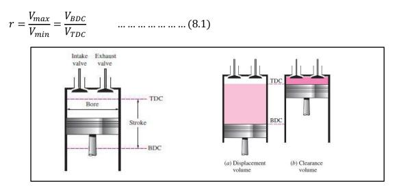
Another term frequently used in conjunction with reciprocating engines is the **mean** effective pressure (*MEP*). It is a fictitious pressure that, if it acted on the piston during the entire power stroke, would produce the same amount of net work as that produced during the actual cycle:
