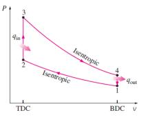
No work is involved during the two heat transfer processes since both take place at constant volume. Therefore, heat transfer to and from the working fluid can be expressed as:
