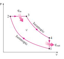
Then the thermal efficiency of the ideal Diesel cycle under the cold-air-standard assumptions is expressed as:
