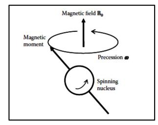
Figure 4: the 1H nucleus processes in an External magnetic field (right).
