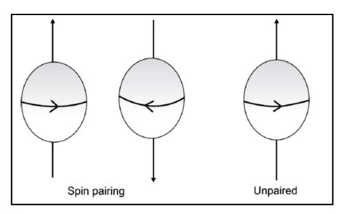
Figure2: Spin pairing in the nucleus, unpaired spins give magnetic moment
