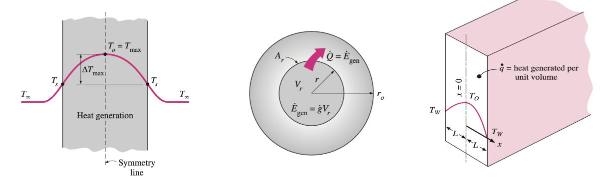
Consider a solid medium of surface area As, volume V, and constant thermal conductivity k, where heat is generated at a constant rate. Heat is transferred from the solid to the surrounding medium at  $T_{\infty}$ , with a constant heat transfer coefficient of h. All the surfaces of the solid are maintained at a common temperature  $T_s$ . Under *steady* conditions, the energy balance for this solid can be expressed as
