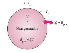
For a large *plane wall* of thickness 2L(As = 2Awall and V=2LAwall), a long solid *cylinder* of radius  $ro(As = 2\pi ro L \text{ and } V = \pi r_o^2 L)$ , and a solid *sphere* of radius  $r0(As = 4\pi r_o^2 \text{ and } V = 4/3\pi r_o^3)$ , Equation reduces to
