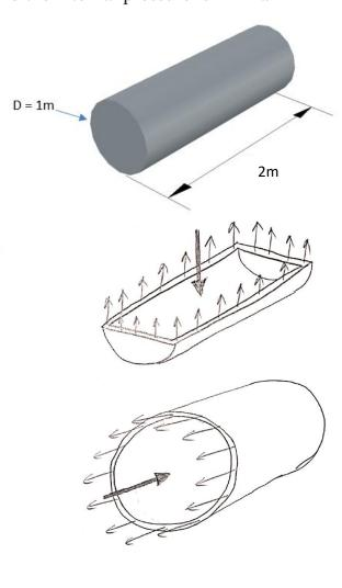
Ex; for the cylindrical tank shown, determine the tangential and longitudinal stress in the wall, the thickness of the wall is 6.4 mm and the internal pressure is 0.9 MPa
