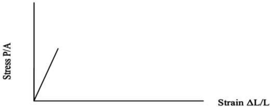
Stress – Strain curve for non ductile material – Cast iron (no plastic deformation)
