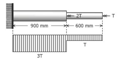
Based on maximum shearing stress  $\tau_{max} = 16T / \pi d^3$ :
