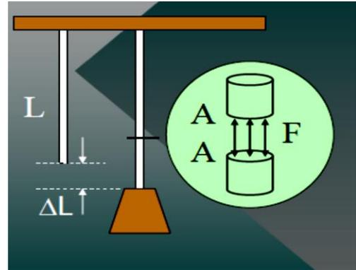
**Example 1.** A steel wire 10 m long and 2 mm in diameter is attached to the ceiling and a (200 N) weight is attached to the end. What is the applied stress?
