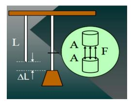
**Example 1**. A steel wire 10 m long and 2 mm in diameter is attached to the ceiling and a (200 N) weight is attached to the end. What is the applied stress? First find area of wire:
