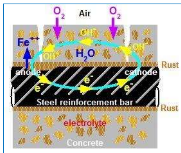
Figure (60): Reinforcement Corrosion progression
