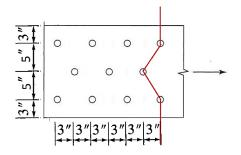
**Example No. 5:** A  $W10 \times 19$  is connected by 8 bolts in webs arranged in two rows as shown in Figure if the section is made from A992, and loaded by tension force (Dead load= 70 kips, Live load= 100 kips). Check the adequacy of the section by using LRFD method. The holes are made for (5/8) in diameter bolts.
