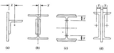
$\bar{x}$ : connection eccentricity, *in*. It is the distance from the center of the section to the place of attachment obtained from the code.
