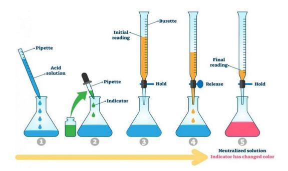
**The equivalence point** : is the theoretical end of the titration where the number equivalents of the analyte exactly equals the number of equivalents of the titrant added
