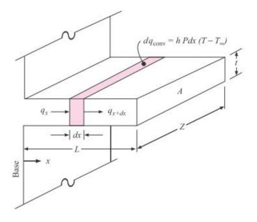
The energy balance on an element of the fin of thickness dx is
