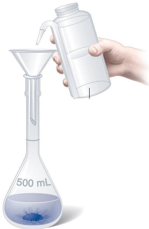
(b) A portion of the solvent is added to the volumetric flask.
