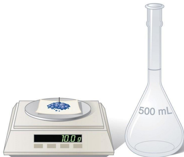
(a) An amount of solute is weighed out on an analytical balance and then
