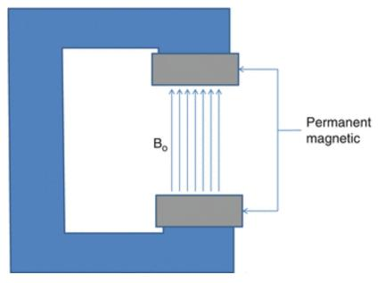
Figure 4: C-shaped permanent magnet
