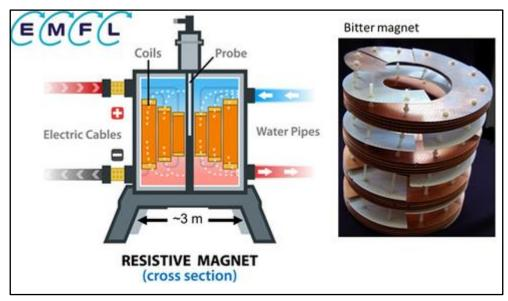
Figure 5: Cross Section of Resistive Magnet.
