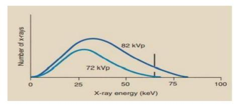
A change in kVp has no effect on the position of the discrete x-ray emission spectrum
