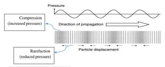
**The frequency of the wave** The number of complete cycles in a unit of time is the frequency (f) of the sound.
