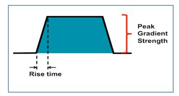
Electrical currents are pulsed on and off during imaging, and gradients typically have a trapezoidal waveform as shown in the diagram above from which various measurements are derived.
