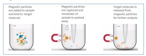
A diagram showing the magnetic bead-based purification protocol. Image credit
