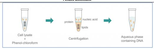
A diagram showing phenol-chloroform extraction steps: adding the phenol-chloroform mixture to the cell lysate, centrifugation, followed by washing with water to obtain the isolated DNA.
