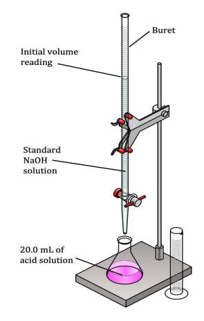
**Principle of Titration:** It is based on the complete chemical reaction between the analyte and the reagent (titrant) of known concentration.
