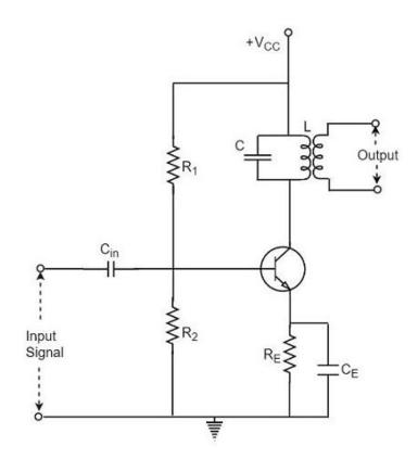
The tuner circuit is nothing but a LC circuit which is also called as resonant or tank circuit. It selects the frequency. A tuned circuit is capable of amplifying a signal over a narrow band of frequencies that are centered at resonant frequency.
