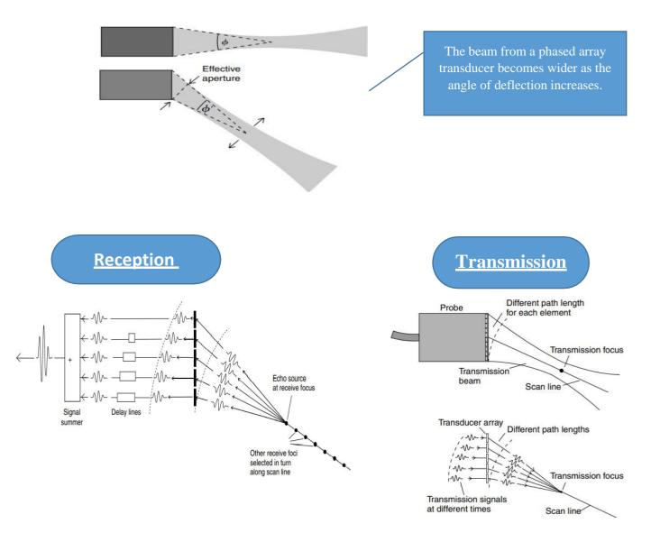
• The principle is the same as for a linear-array transducer, except that the receive foci lie along a scan line that is generally oblique.
