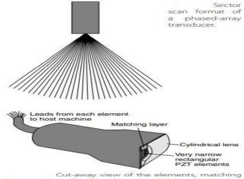
Cut-away view of the elements, matching layer and lens of a phased-array transducer.
