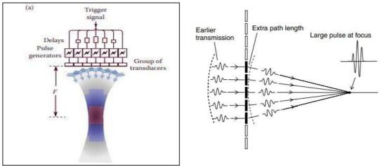
For linear-array transducers, focusing in transmission requires that pulses from all the elements arrive simultaneously at the transmission focus, in order to concentrate the power into a narrow 'focal zone'.
