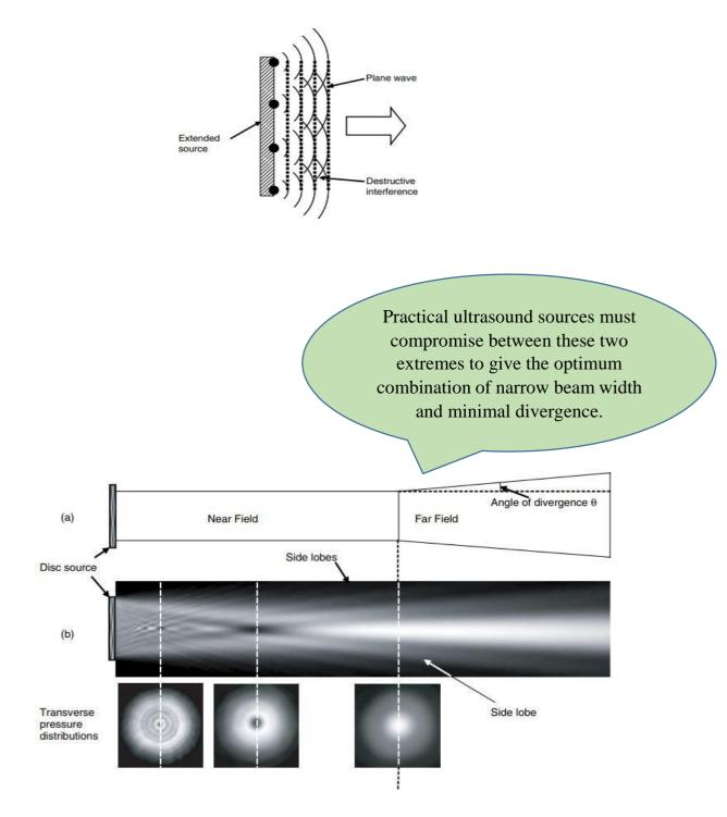
The basic shape of the ultrasound beam produced by a plane disc transducer is illustrated in Figure above, it can be divided into two parts. These are :
