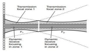
Further improvement in lateral resolution, For example, the operator might select transmission foci at two different depths - F 1 and F 2
