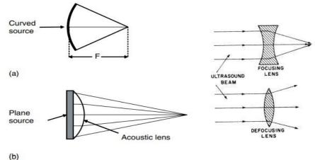
The curved source (Figure above) is manufactured with a radius of curvature of F and hence produces curved wave fronts which converge at a focus F cm from the source.
