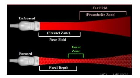
The focusing effect on a beam is strongest when the focal length F is short in relation to the near-field length of a similar unfocused transducer Here, the waves converge rapidly to a very narrow beam width at the focus then diverge rapidly again beyond that point.
