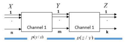
For the series information channel, the overall channel capacity is not exceed any of each channel individually.
