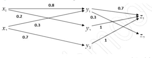
$$p(Y|X) = \begin{bmatrix} 0.8 & 0.2 & 0 \\ 0.3 & 0 & 0.7 \end{bmatrix}, \qquad p(Z|Y) = \begin{bmatrix} 0.7 & 0.3 \\ 1 & 0 \\ 1 & 0 \end{bmatrix}$$
