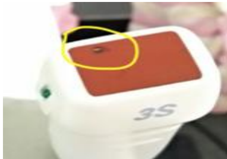
Bubble or crack in ultrasound probe lens
