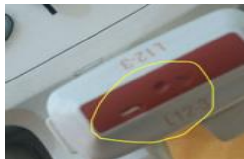
Lens damage with bubbles in ultrasound probe
