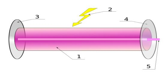
The *optical resonator*, or *optical cavity*, in its simplest form is two parallel mirrors placed around the gain medium, which provide <u>feedback</u> of the light. The mirrors are given <u>optical coatings</u> which determine their reflective properties. Typically, one will be a <u>high reflector</u>, and the other will be
