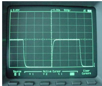
Fig. 10: Capacitor Voltage in Series RC Circuit.
