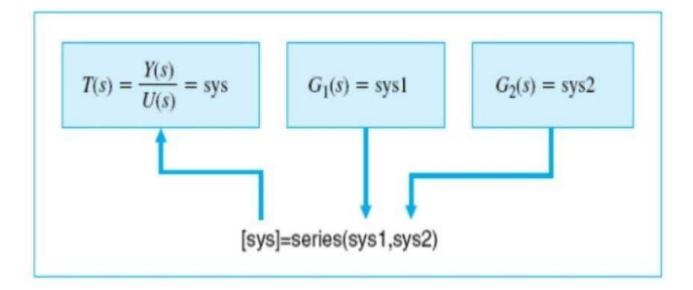
**Example 3:**Given the transfer function of individual blocks generate the system transfer function of the block combinations.
