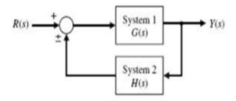
a non-unity feedback system is implemented in MATLAB using the same "feedback" command as shown:
