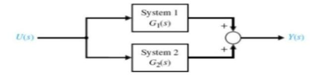
The MATLAB command for implementing a parallel configuration is "parallel" as shown blow:
