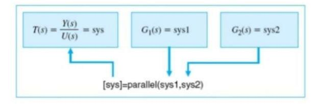
**Example 4:** for previous system defined, modify the MATLAB command to obtain the overall transfer function when the two blocks are in parallel
