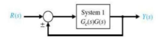
The MATLAB command for implementing a feedback configuration is "feedback" as shown blow:
