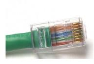
the wires the RJ-45 cable is crimp
