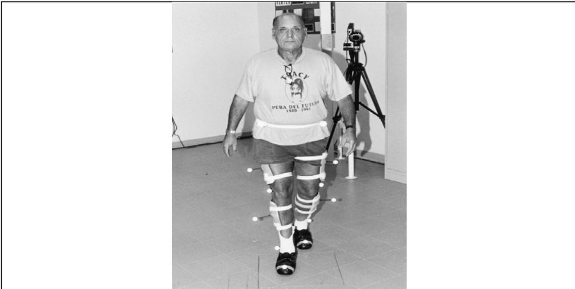
**Figure 3:** This individual is wearing reflective spheres. An infrared camera system can track limb segment motion as the patient walks across the field of view.
