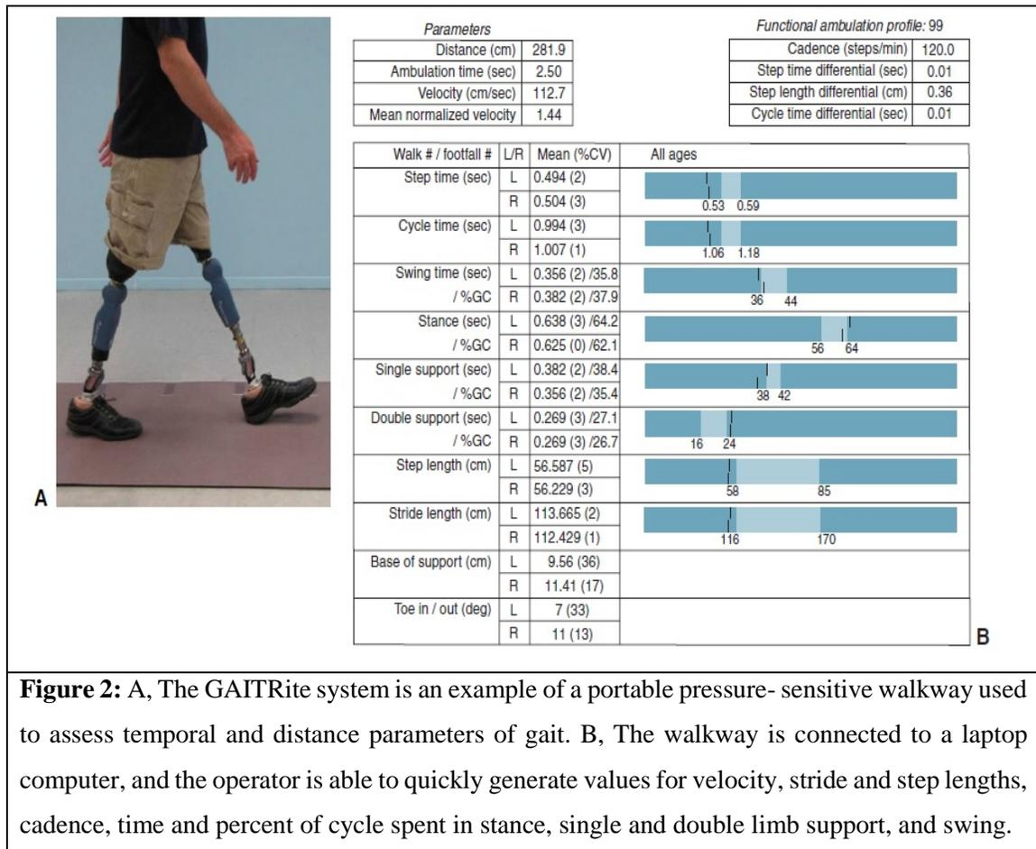
**Figure 2:** A, The GAITRite system is an example of a portable pressure-sensitive walkway used to assess temporal and distance parameters of gait. B, The walkway is connected to a laptop computer, and the operator is able to quickly generate values for velocity, stride and step lengths, cadence, time and percent of cycle spent in stance, single and double limb support, and swing.
