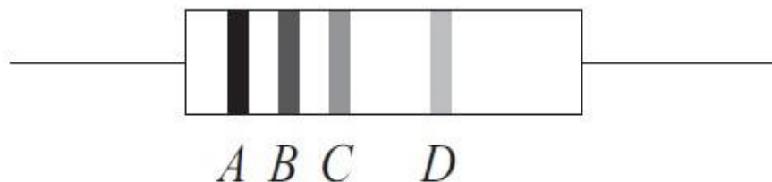
Figure3 : Resistor Color Code
