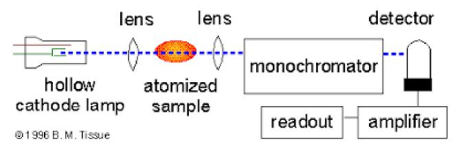
**Component of Atomic absorption spectroscopy**
