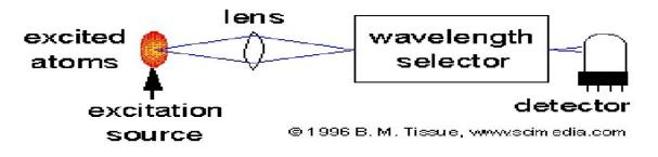
Inserting the sample and subjecting it to high pressure with oxygen, the sample will turn into aerosol and be of a high energy level and then exposed to a flame and these high energy atoms will return to the normal energy level and emit energy in the form of photons.
