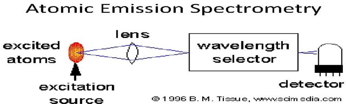
Inserting the sample and subjecting it to high pressure with oxygen, the sample will turn into aerosol and be of a high energy level and then exposed to a flame and these high energy atoms will return to the normal energy level and emit energy in the form of photons.
