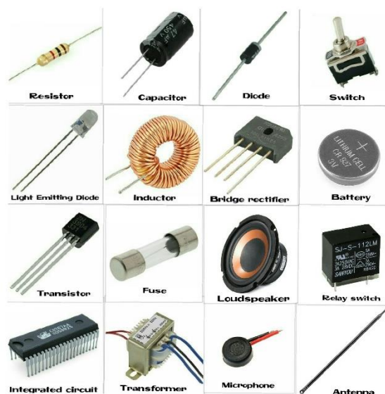
Picture (1) Electrical components.
