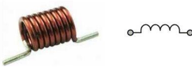
Picture (3) The electrical coil.
