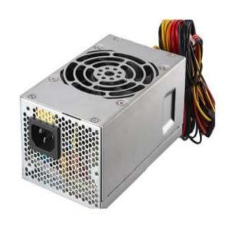
3.3 volt for micro chips (processor or controller).
