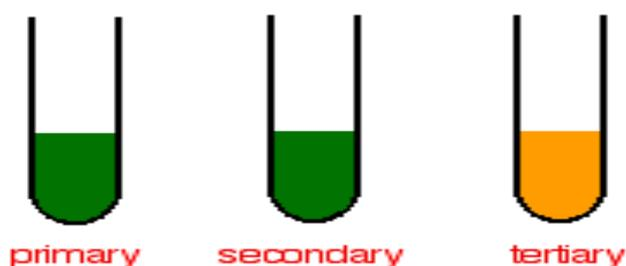
In the case of a primary or secondary alcohols, the orange solution turns green. The Schiff's test will need to be performed to distinguish between the primary and secondary alcohols. With a tertiary alcohol, there is no color change.
