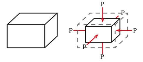
If the forces acting on an object deform it in such a way that there is a change to the volume of that object, then we are talking about volumetric stress.
