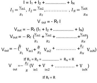
$$V_{out} = - (V_{in1} + V_{in2} + \dots + V_{inN})$$
