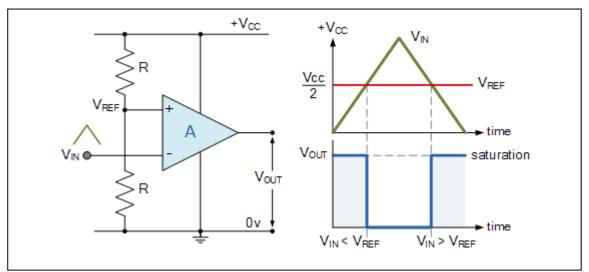
8.2. Positive Voltage Comparator (non-inverting) circuit detects when the input signal V<sub>in</sub> is ABOVE or more positive than the reference voltage then the circuit produces an output at V<sub>out</sub> which is HIGH as shown.
